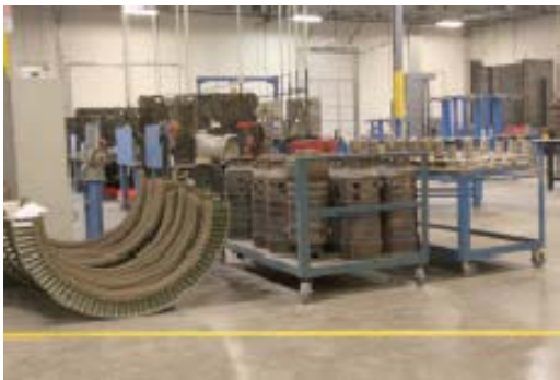
A1. Standing inventory of 501AA diaphragms, DF42 baskets for Westinghouse engines, and 501B fuel nozzles (left to right) A2. Phoenix Turbine's new combustion repair and manufacturing cell (right)
